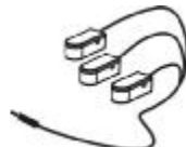
Infrared Extender X 3 1,1.5,2m in length
