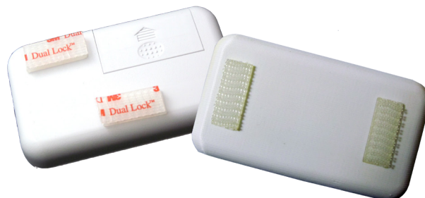
Figure 4 – Remove backing from Dual Lock strips
