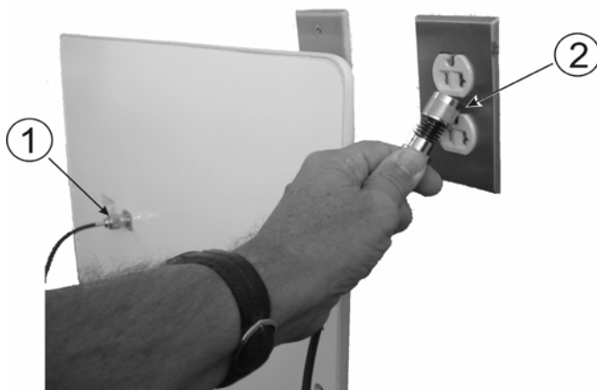
Figure 26 Short Load to Earth Ground
