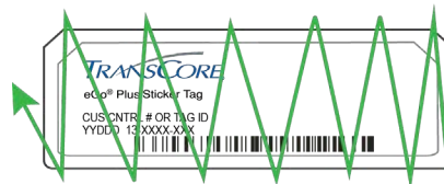
Figure 13 Rub Tag to Bond Adhesive to Windshield
