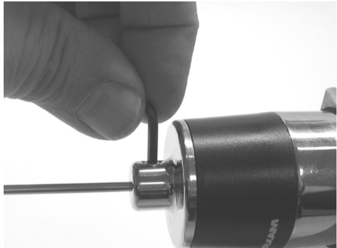
**Figure D-6 Lower and Upper Hex Screws**
