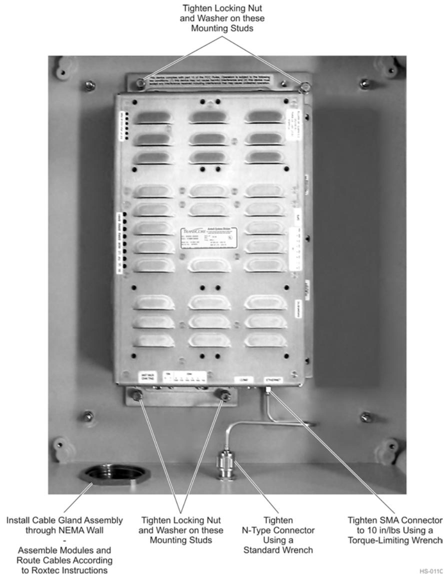
**Figure 3-9 Encompass Reader Mounted in a NEMA Enclosure**
