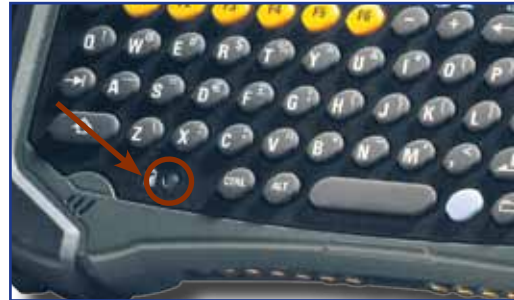
Battery Status indicator on CE8640B
