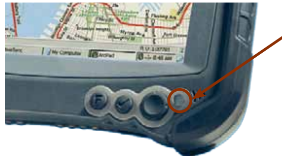
Battery Status indicator on CE8800B
