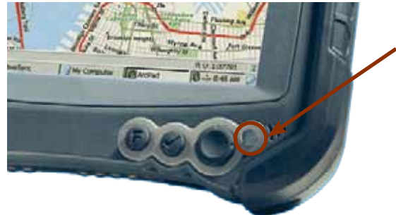
Battery Status indicator on CE8800B
