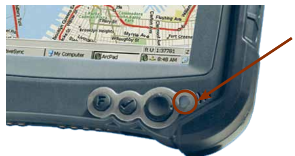
Battery Status indicator on CE8800B
