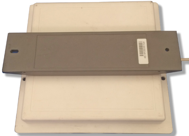
Figure 22 Tag and Antenna Orientation (horizontal polarization)
