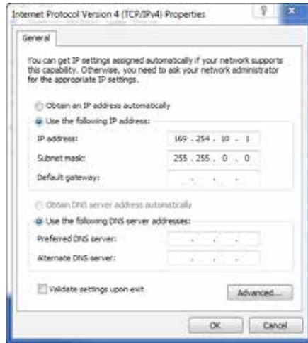
Figure 15 Connecting Directly to Computer Ethernet Port
