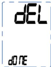
Note: To exit out of delete mode without deleting any records, press START/STOP button before pressing "S" to confirm any delete commands.
