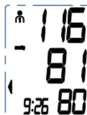
2. This device will proceed to data transmission after measurement. The Bluetooth symbol blinks on the LCD indicates data is transmitting.
