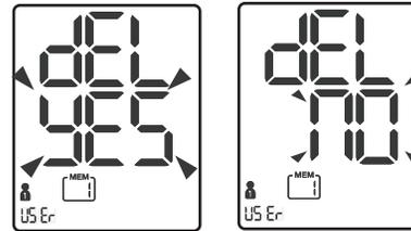
3. Press "START/STOP" button to confirm delete the records, the display will show "User ID + dOne" and then the monitor will turn off.
