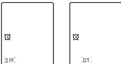
2. When you choose turn on, press "START/STOP" button, the LCD will display the time. Choose "MEM" or "SET" button to set the time, press "START/STOP" button to confirm, the LCD will display "dOnE" and then the monitor will turn off.
