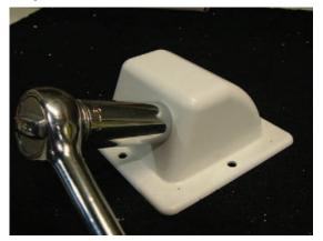
Tighten using a ¾" wrench or socket. Tighten until the Cable Lock touches the Boot as shown in Step 3.
