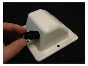
Attach Ethernet Cable Lock on side of the Ethernet Boot. This is easiest to do before you attach the RJ-45 Jack.
