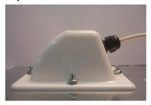
Place the Ethernet boot over the 4 Screw Posts. Apply 4 Kept nuts to the screw posts and tighten until the gasket makes full contact with the Ethernet boot. The gasket should be at least 50% compressed.
