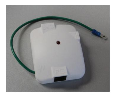
Connect the power adapter to the power socket on the Power over Ethernet Adaptor (POE), and plug the other end of the power into an electrical outlet. Plug the RJ-45 Cable from the unit into the POE. The Station Adaptor will be powered on and the power indicator on the top panel will turn on.
