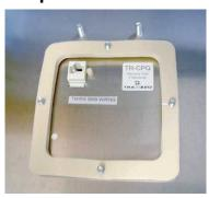
Remove gasket backing and place boot cover on radio. This will ensure that you attach the sticky side of the gasket to the underside of the Ethernet Boot. Make sure the Gasket is free of gaps.
