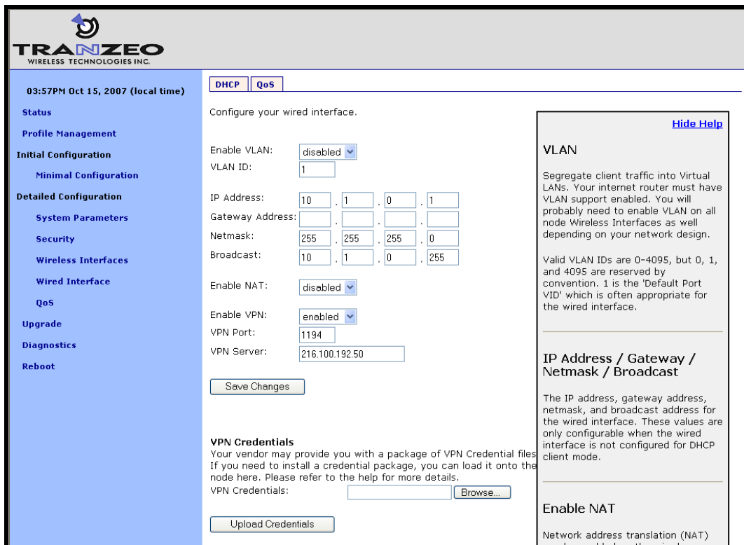
Figure 56. Configuring VLAN for Ethernet interface
