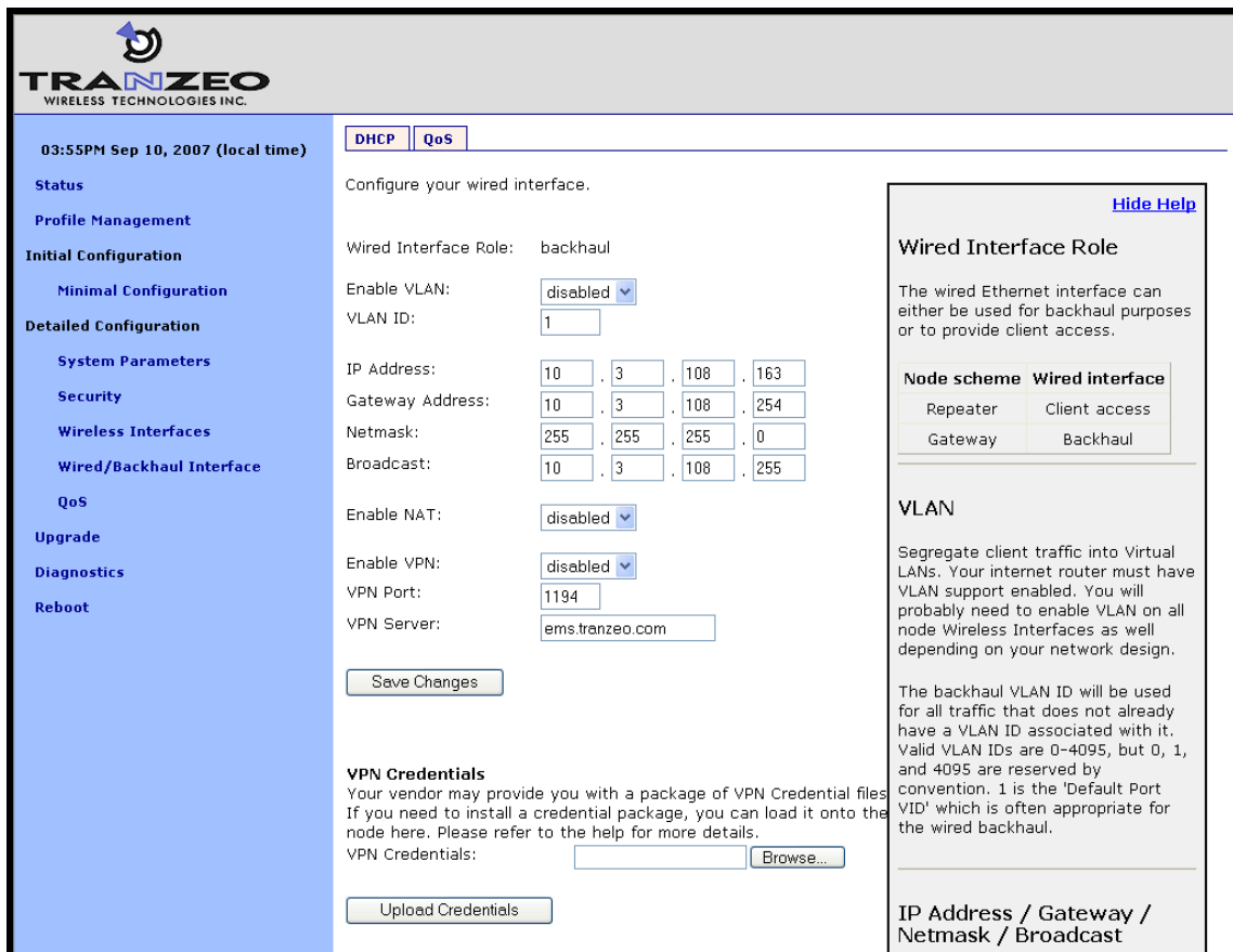
Figure 58. Configuring VLAN for backhaul interface
