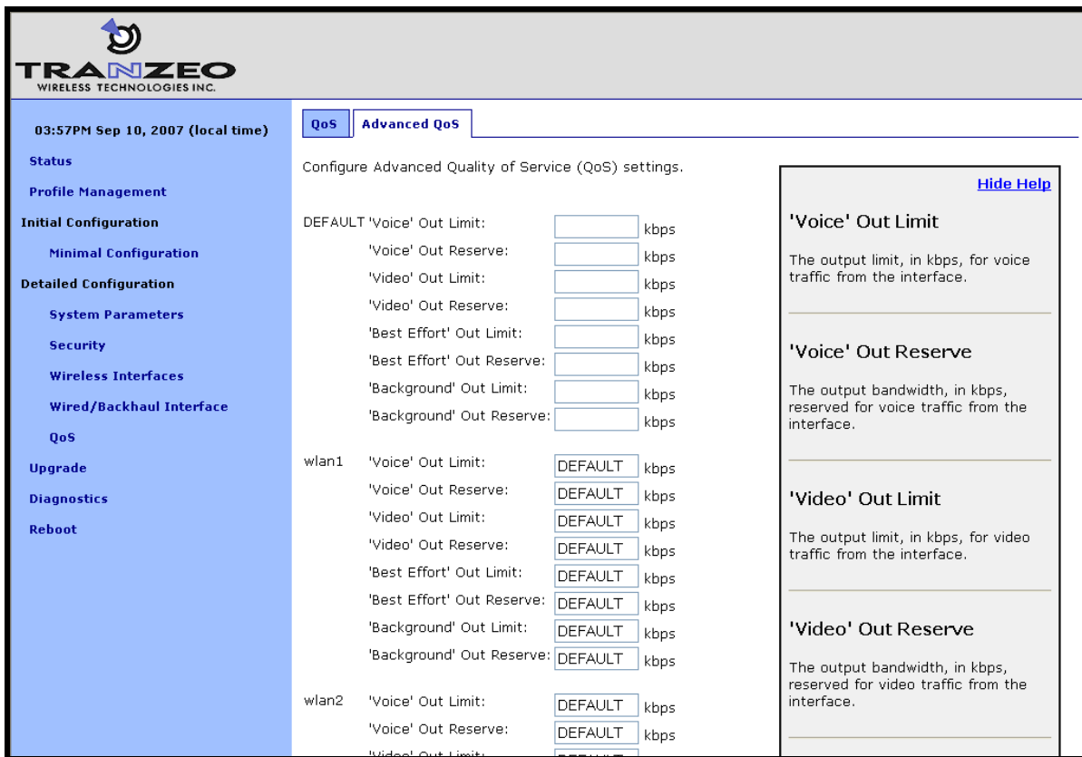
Figure 54. Advanced QoS configuration (only settings for some interfaces are shown)
