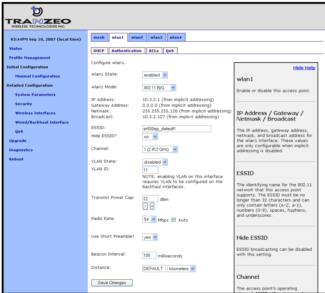
Figure 42. Access point interfaces
