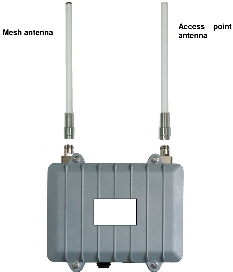
Figure 5. Connecting the mesh and access point antennas
