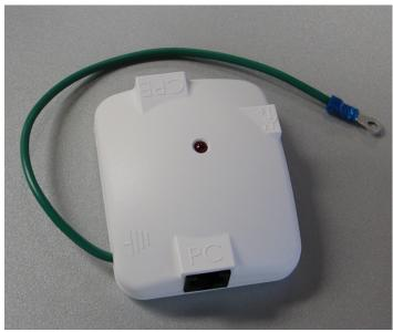
Connect the power adapter to the power socket on the Power over Ethernet Adaptor, and plug the other end of the power into an electrical outlet. Plug the RJ-45 Cable from the unit into the POE. The Station Adaptor will be powered on and the power indicator on the top panel will turn on.
