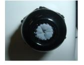
If you are not going to be using the second port make sure that it is tightened down to ensure a weather-tight seal.
