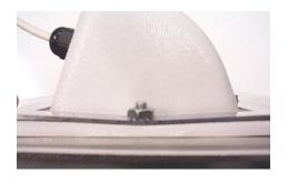
This is an example of over tightening. Over tightening connections like this may crack the boot and will compromise the gasket seal. Over tightening is not covered by warranty.
