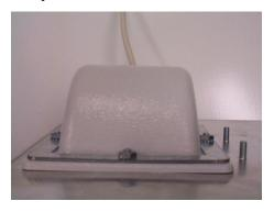
Place the Ethernet boot over the 4 Screw Posts. The screws should just barely clear the tightening bracket. Apply 4 Keep nuts to the screw posts and tighten until the gasket makes full contact with the Ethernet boot. Do not over tighten.
