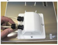
Insert the Cat 5 Cable and tighten the Boot Cover. Be sure to pull enough cable through to reach the RJ-45 connector with an RJ-45 jack attached. The Gasket must be attached to the Boot so that it sits between the radio and the boot.
