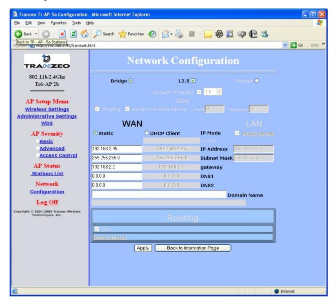
This page allows you to control the network configuration of the device. Enable the Router option to change the IP configuration for the LAN. You can also choose Static or DHCP IP configuration for both the device and any associated IP clients.
