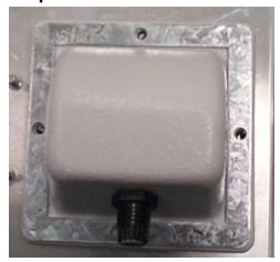
Attach optional tightening bracket on top of the Ethernet Boot. This is easiest to do before you attach the CAT 5 cable. The Gasket must be attached to the Boot so that it sits between the radio and the boot.
