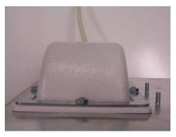
Place the Ethernet boot over the 4 Screw Posts. The screws should just barely clear the tightening bracket. Apply 4 Ket nuts to the screw posts and tighten until the gasket makes full contact with the Ethernet boot. Do not over tighten.
