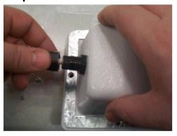
Insert the Cat 5 Cable and tighten the Boot Cover. Be sure to pull enough cable through to reach the RJ-45 connector with an RJ-45 jack attached. Attach tightening bracket on top of the Ethernet Boot. This is easiest to do before you attach the CAT 5 cable. The Gasket must be attached to the Boot so that it sits between the radio and the boot.
