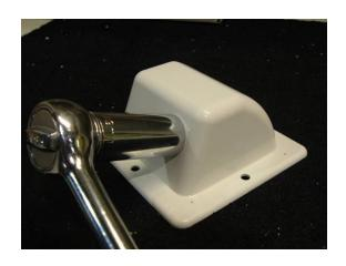
Tighten using a ¾" wrench or socket. Tighten until the Cable Lock touches the Boot as shown in Step 3. USE HAND TOOLS ONLY. DO NOT OVERTIGHTEN as you may damage the environment seal.
