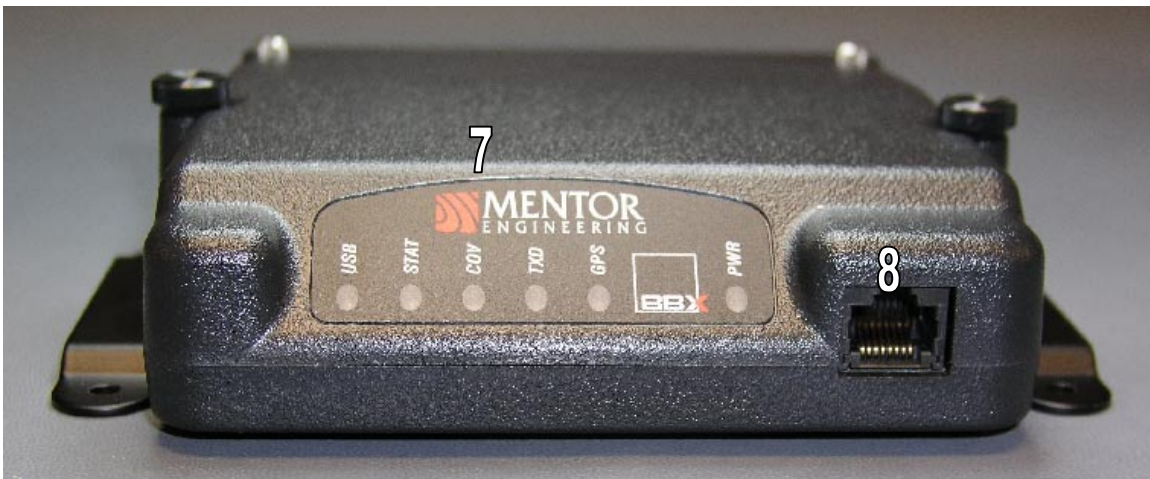
Figure 3: BBX Interface points (Front View)
