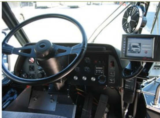
Ranger Installed in an Orion II Bus
