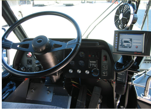
Ranger Installed in an Orion II Bus
