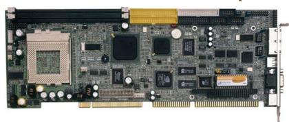
The HS-6038 is a 133MHz FSB Intel<sup>®</sup> 82815/82801BA chipset-based board designed for PICMG Bus Celeron<sup>™</sup>/Coppermine<sup>™</sup>/Tualatin<sup>™</sup> 800MHz~1.2GHz CPU compatibility. These features combine and make the HS-6038 an ideal all-in-one industrial single board computer. Additional features include an enhanced I/O with CompactFlash, VGA, dual LAN, audio, and two COM interfaces.
