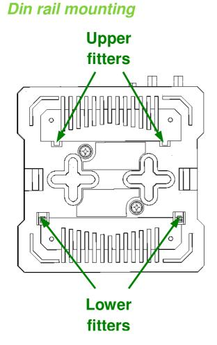
Make enough space for Zipabox on your Din-rail. Hook upper fitters on the back of your Zipabox to the Din rail and press Zipabox slightly to snap lower fitters.
