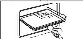
Adjust the grid and grill pan runner position to allow for different heights of food.
