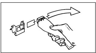
To correctly locate the grill pan on the shelf, ensure that the cut out on the underside of the handle bracket locates over the front bar of the shelf.
