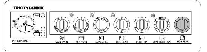
To operate the hotplates turn the control knobs in either direction to vary the heat setting. The highest number represents the hottest setting and the lowest the coolest setting.
