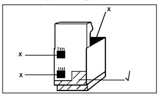
To move the cooker, open the main oven door and lift the cooker by holding the inside top of the compartment.
