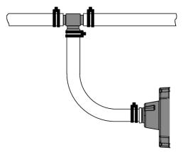
For aircraft with  $\frac{1}{4}$  inch static lines, two adapters are provided which can convert from  $\frac{1}{4}$  inch inside diameter hoses to the 5 mm hose in the install kit.
