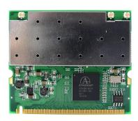
DNMA-83 is a 802.11n a/b/g wifi 3x3 mini-PCI module designed specifically to enable high-performance 3x3 MIMO access point (AP) and router solutions for dual-band (2.4/5GHz) applications that demand robust link quality and maximum throughput and range. Setting new standards in throughput, range, reliability, and power consumption, DNMA-83 delivers the ultimate wireless triple play experience for video, voice, and data transmission in the home, for the business, and on the road.
