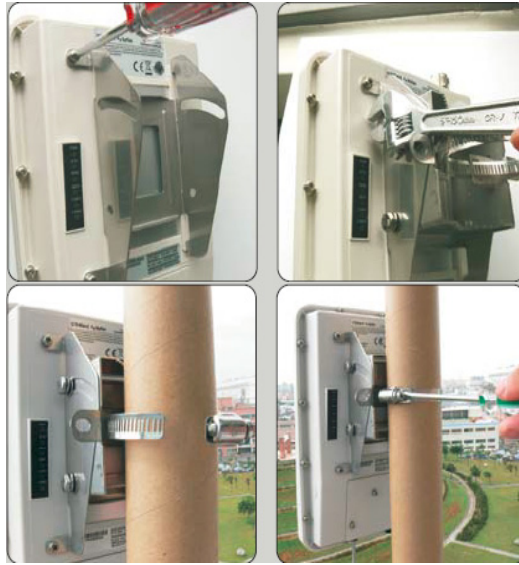
Figure 3-5. Attaching the SecureMesh Connector
