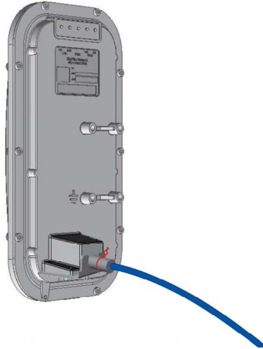
Figure 3-3. Attaching tie wraps to the gasket neck
