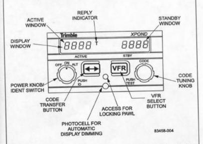
The active code is displayed on the left side of the display window and the standby code is displayed on the right side. The transponder displays a "T" (reply indicator) to the right of the active code when it responds to an interrogation from a ground station indicating that the aircraft is being seen on radar. The "T" also verifies proper operation when using the self-test feature.
