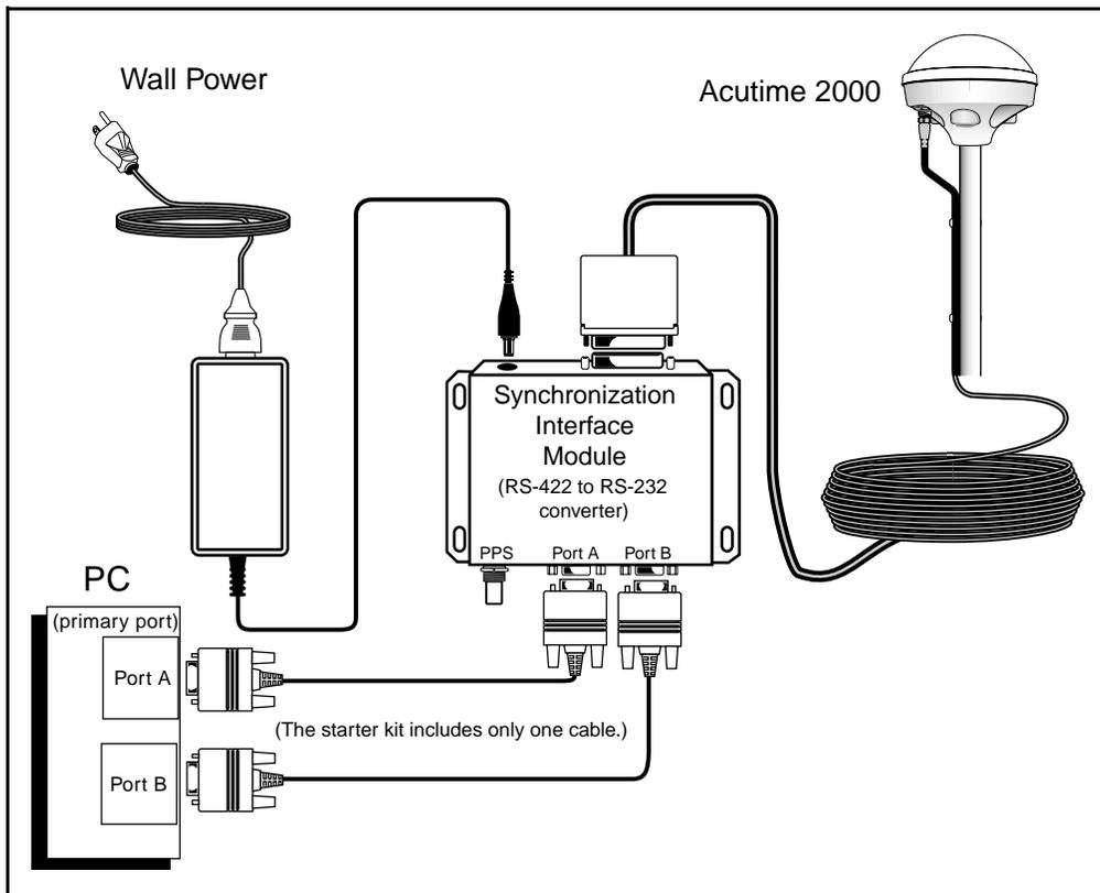
**Figure 2-1 Connection Diagram**
