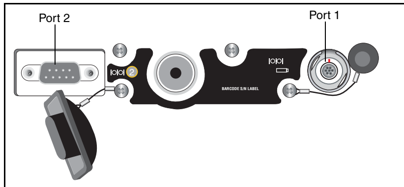
Figure 19.1 Trimble R8 serial ports
