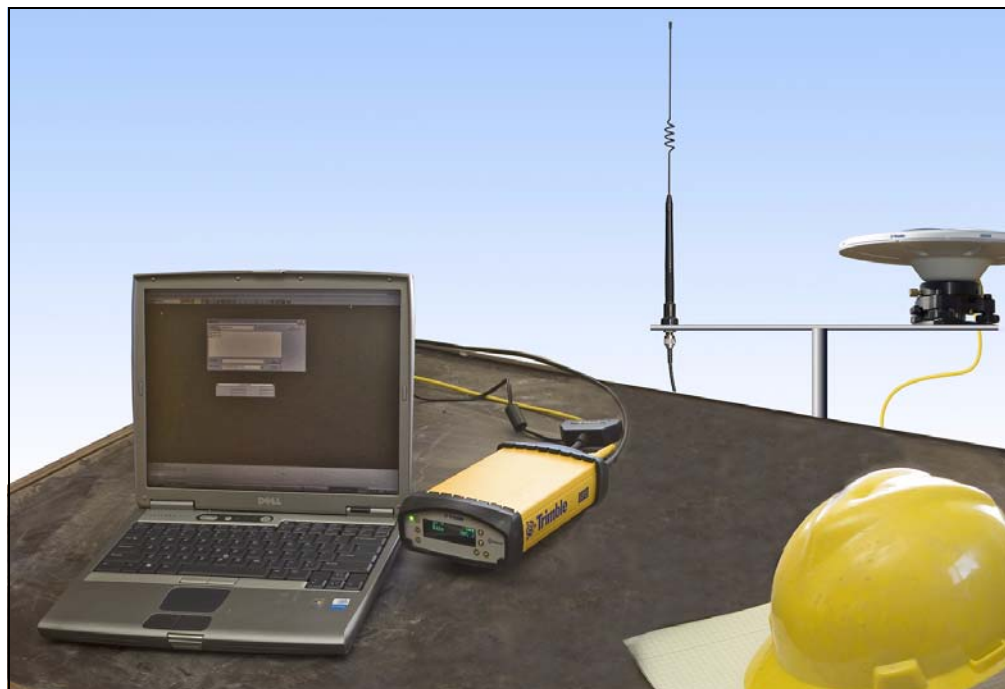
Figure 5.1 SPSx50 receiver permanent installation
