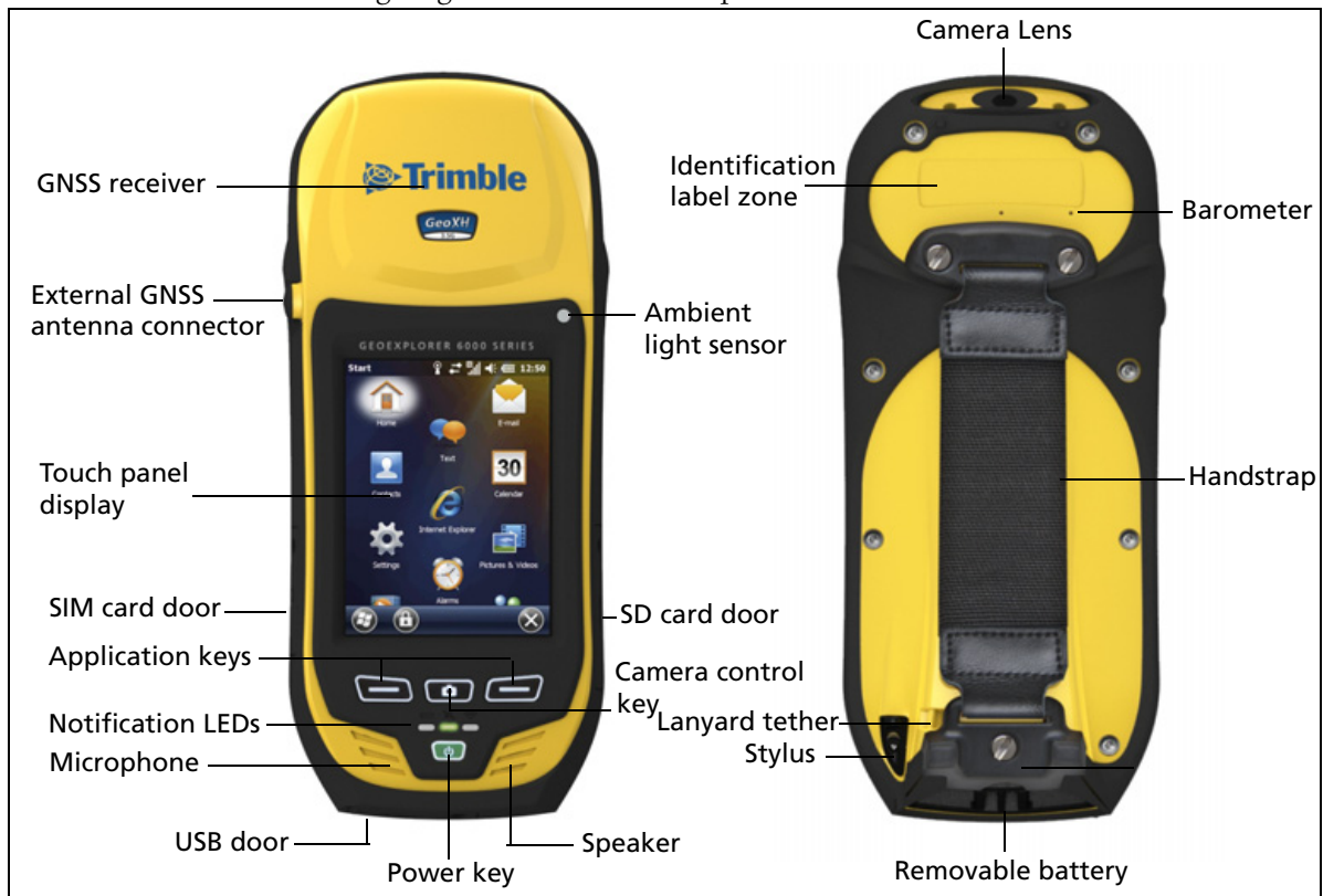
Figure 2.1 Parts of the GeoExplorer 6000 series handheld
