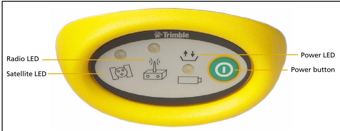
Figure 2.2 Front panel of the SPSx80 Smart GPS antenna
