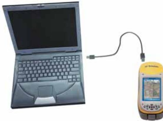
Figure 4.1 Connecting the handheld to a computer using the USB data cable
