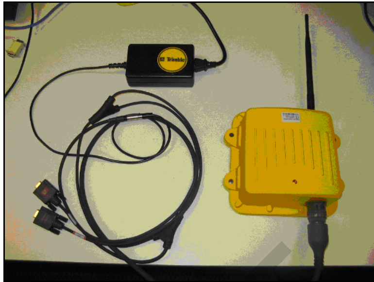
Figure 3.1 Radio service cable
