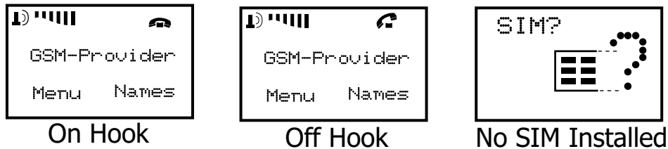
Figure B-3 Start Screen Elements
