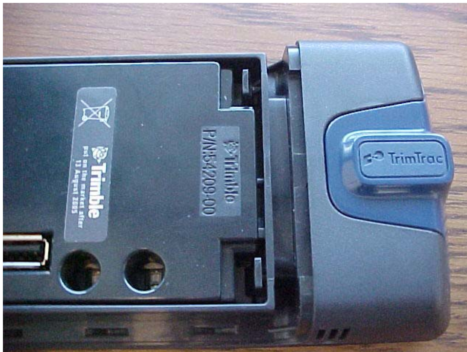
Figure 32. Provisioning Module Improperly Inserted. Upper Tab not Latched Properly.
