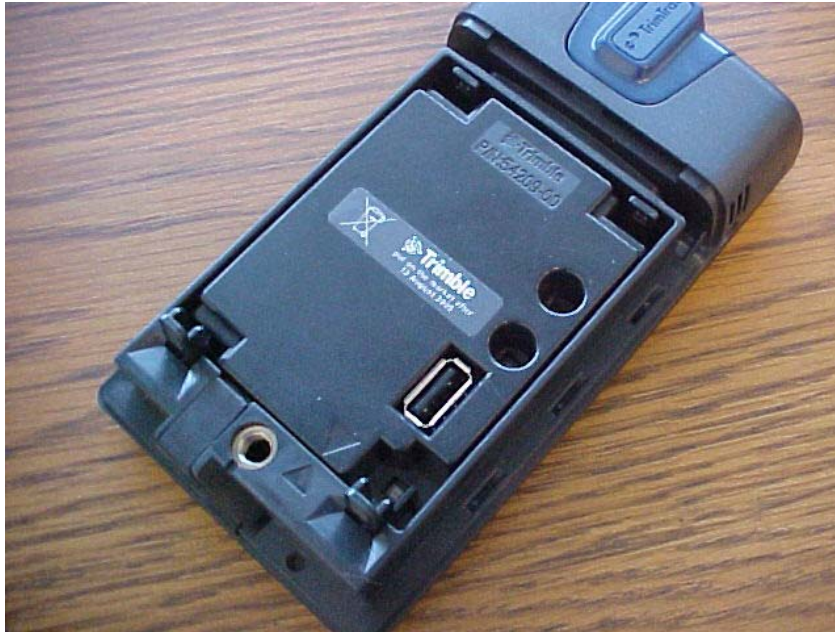
Figure 3. Provisioning Module inserted into a TrimTrac ProE
