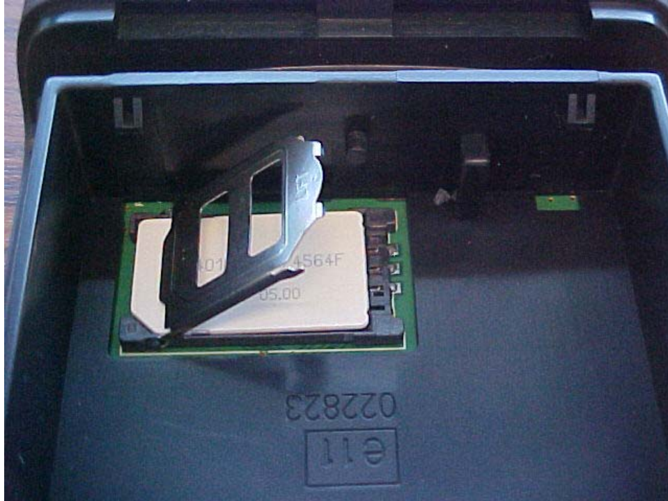
Figure 29. Open SIM Card Holder.
