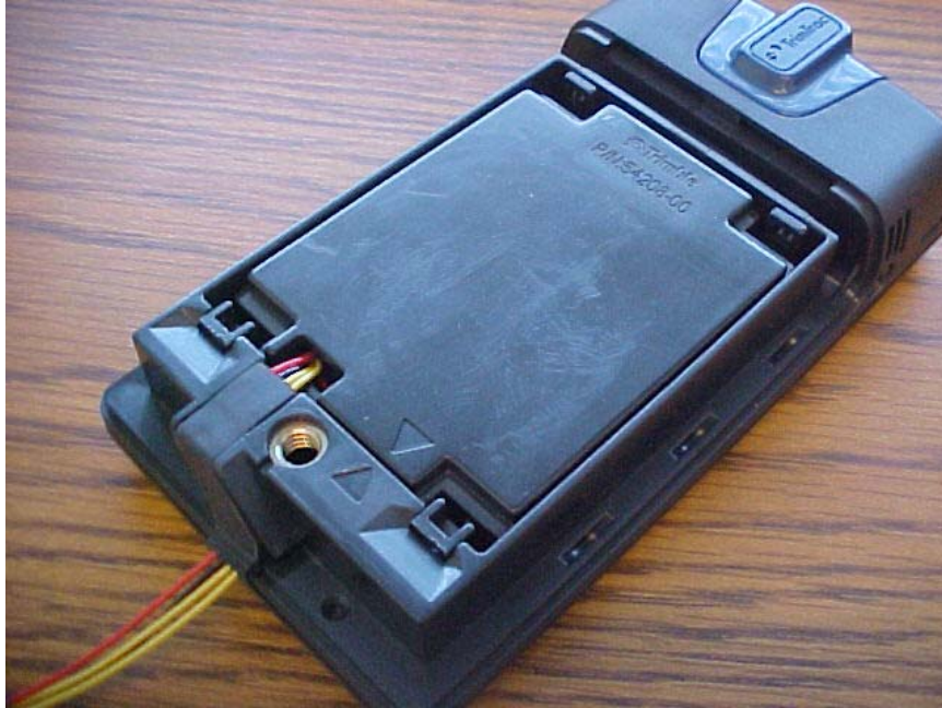
Figure 4. Vehicle Adapter Module inserted into a TrimTrac ProE
