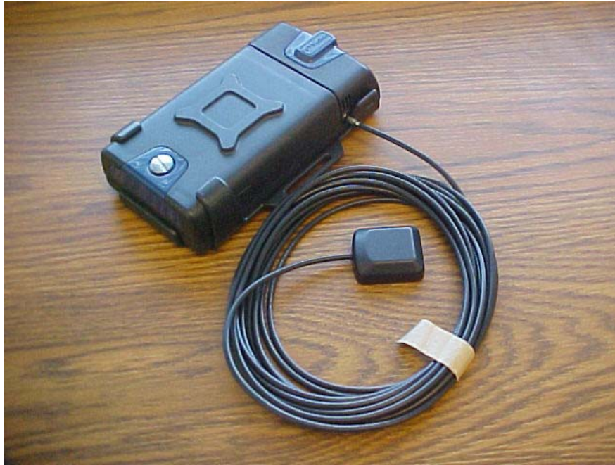
Figure 19. External GPS Antenna Connected to TrimTrac ProE
