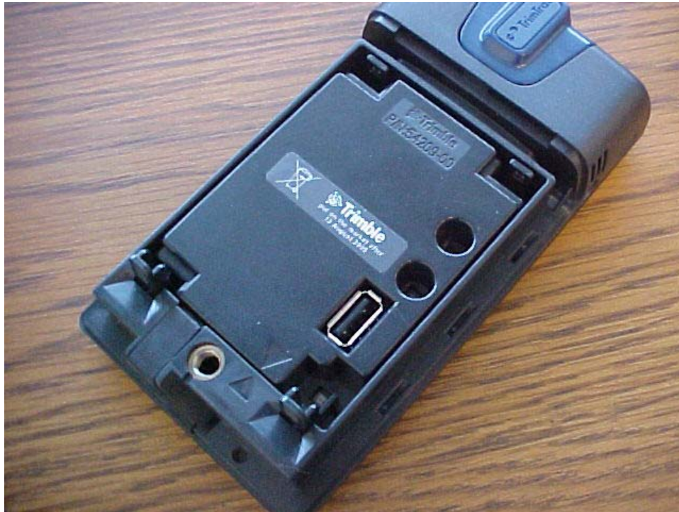
Figure 31. Properly Inserted Provisioning Module.
