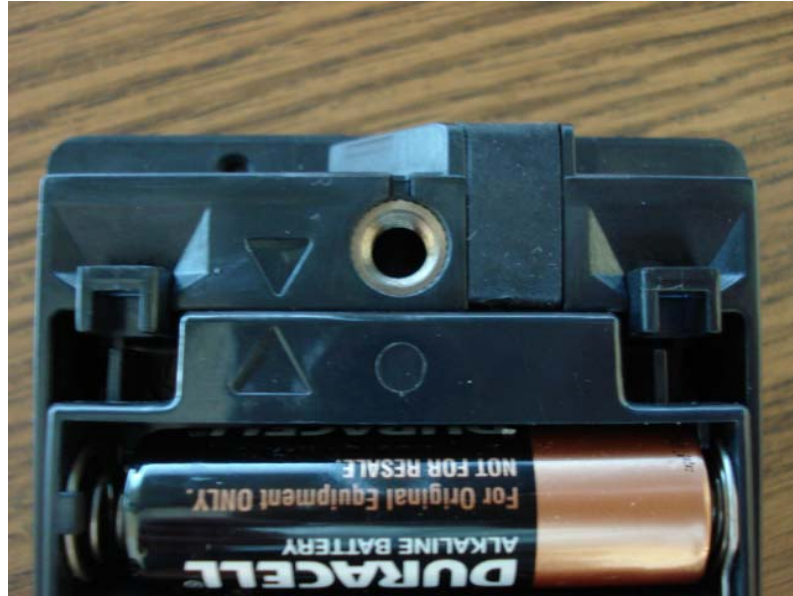
Figure 11. Align Arrows on base and module.
