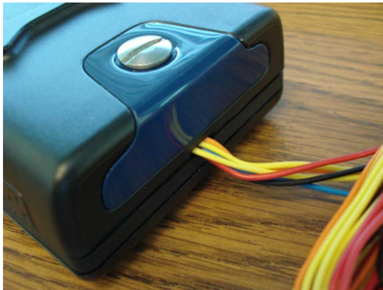
Figure 16. Cover in place with Wires Properly Routed
