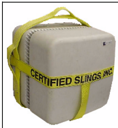
Figure 4-3: IFU Correctly Positioned in an IFU Sling (Front View)
