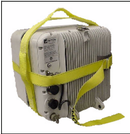
Figure 4-4: IFU Correctly Positioned in an IFU Sling (Rear View)
