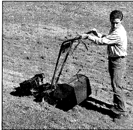
Figure 4-3: Raise tines off ground and look behind when moving in reverse.
