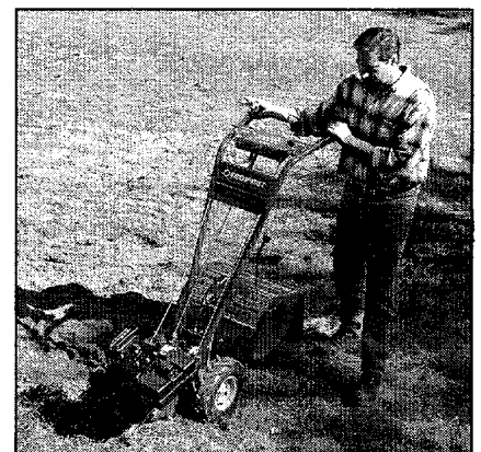
Figure 4-5: With tiller balanced over wheels (and tines out of the ground), push handlebars sideways to turn tiller.
