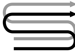
Figure 10: Use an overlap technique on every pass.
