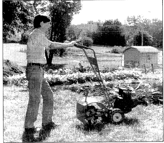
Photo 4-5: Lining up the tiller to enter the next row.
