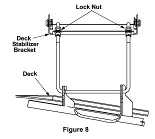
Locate the two lock nuts on the opposite side of the stabilizer bracket. See Figure 8. Tighten the lock nuts to raise the front of the deck; loosen the lock nuts to lower the front of the deck.
