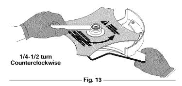
9. Remove the locking rod from the locking rod slot.
