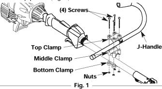
While holding the three pieces together, install the four (4) screws through the top clamp and into middle clamp.
