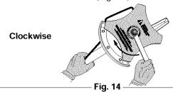
Remove the nut, blade retainer and blade. Store the nut and blade together for future use in a secure place. Store out of children's reach.
