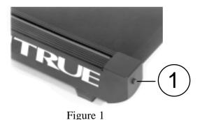
·Turn both rear roller adjustment bolts (Detail 1) counter-clockwise until treadbelt just begins slipping when walking on it, then turn both rear roller adjustment bolts clockwise in equal quarter turn increments until treadbelt stops slipping. NOTE: Be sure to run on treadbelt to ensure that the treadbelt does not slip while under load.
