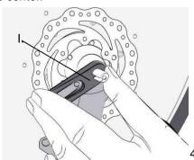
2. To place the M. disc brake on the power wheel (A side) to be locked by M. screw (Disc brake is optional)
