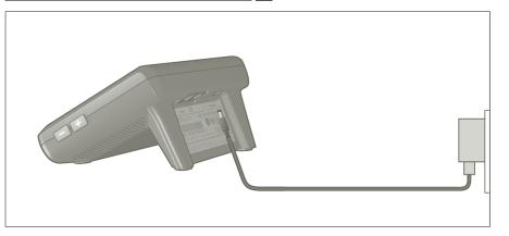
Connect the power supply adapter to RTX3370 and to an electrical outlet. The display of the RTX3370 will light up when the system is ready for use.
