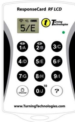
The ResponseCard RF LCD keypad is handheld designed to send responses over RF to a receiver.
