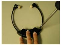
Remove the two screws located on the back of the headset.
