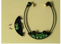
Turn the headset over and remove the faceplate with the logo and batteries attached.
