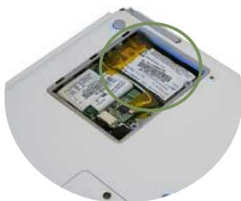
5. Carefully, slide the card out of the slot. Be sure to unscrew the antenna leads from the card before fully removing the card from the interior of the compartment.
