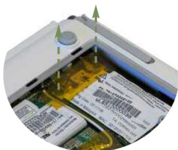
6. Take the new wireless networking card you obtained from your dealer and carefully align it into the connector slot. Attach the antenna leads to the card before inserting it fully into the compartment.
