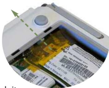
7. Once the leads are connected, press downward on the card to push it into position and replace the screws to hold the card in place.
