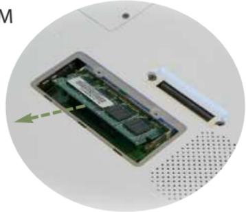
6. To insert a new RAM module, align the connector pins on the bottom of the RAM module with the RAM module socket and slide the module into the socket. Once properly inserted in the socket, press the RAM module down until it clicks into place.
