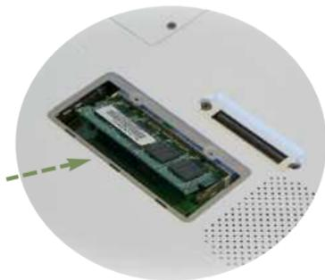
7. Replace the cover on this compartment and then replace and tighten the screws.
