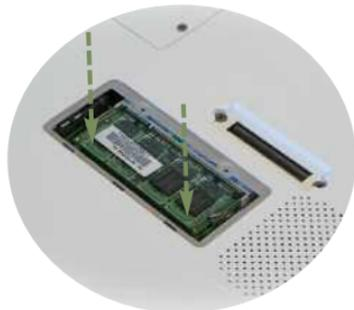
**NOTE:** Your Sahara Slate PC supports dual channel RAM. In order to take advantage of this higher bandwidth feature, you'll need to install a memory module that matches the primary module installed on the other side of the motherboard at the factory. Check with your dealer if you are unsure what module your system currently has installed.
