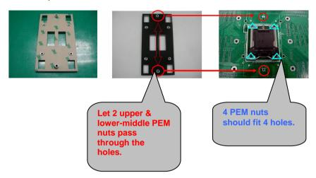
Locate four screw holes on socket and screw the socket to the PCB board.
