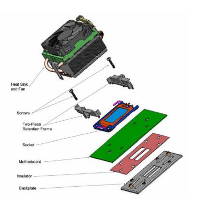
Figure 1. Detailed View of the Thermal Solution AMD PIB Platforms based on the AMD Socket F Processor
