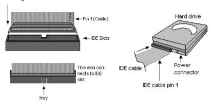
Simply plug in the BLUE END of the IDE cable into the motherboard IDE connector, and the other end into the drive. Each standard IDE cable has three connectors, two of which are closer together. The BLUE connector that is furthest away from the other two is the end that connects to the motherboard. The other two connectors are used to connect to drives.
