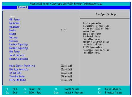
The system displays advanced details like the number of heads/cylinders/sectors on the detected disk and the maximum storage capacity of the disk.
