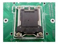
NOTE: Do not assemble CPU before securing socket with screws.
